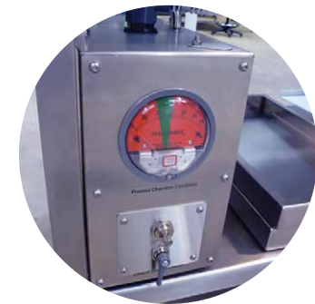
Manual Needle Valve controlled compressed air venturi
