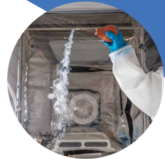
Unidirectional airflow maintained between 0.36 and 0.54m/s
